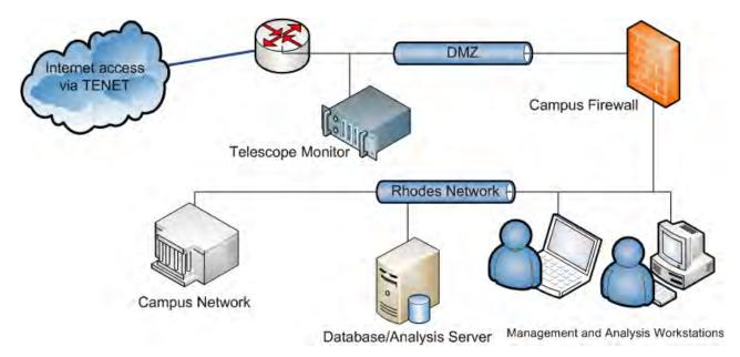
Figure 3.1: Rhodes Network Telescope System
